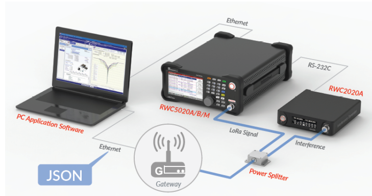
Fig 3.24 The Concept of non-regression test of gateways
